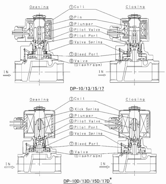
\* The structure differs slightly for DP-12/14/16/18/12D/14D/16D/18D.
