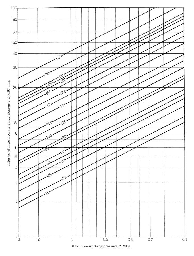
Fig.2 Maximum interval of intermediate guide elements according to the nominal pipe diameters
