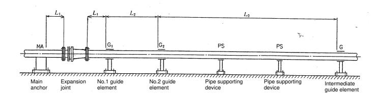
Fig.1 Mounting intervals of guide element
